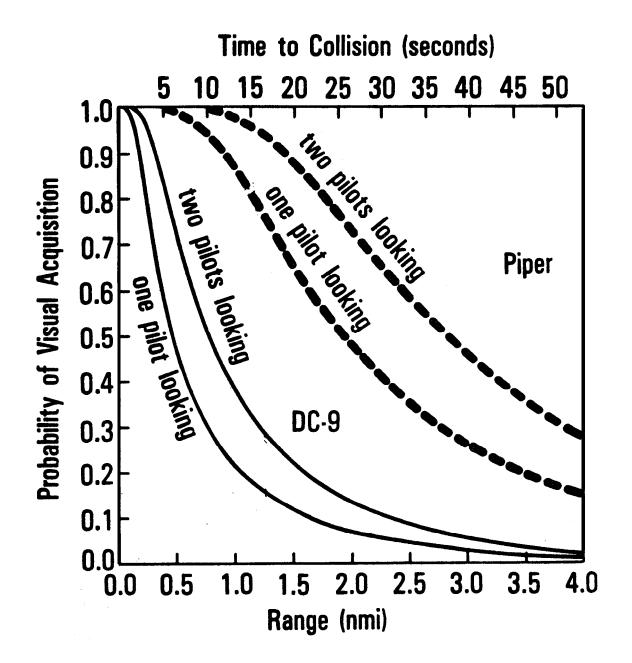
Figure 3.--Probability of seeing the other aircraft as a function of time until collision.
