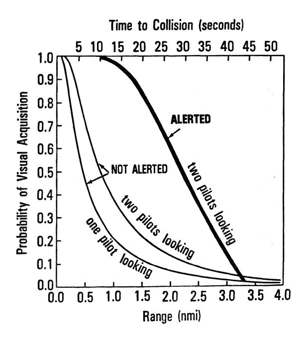
Figure 4.--The effect of **TCAS-type** alert on the **prob**ability that the DC-9 pilot would see the Piper Aircraft.
