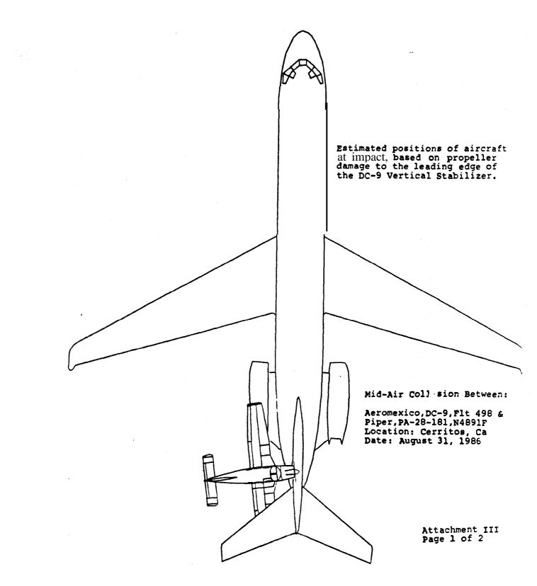
Figure 6.--Collision geometry as viewed from above the DC-9.
